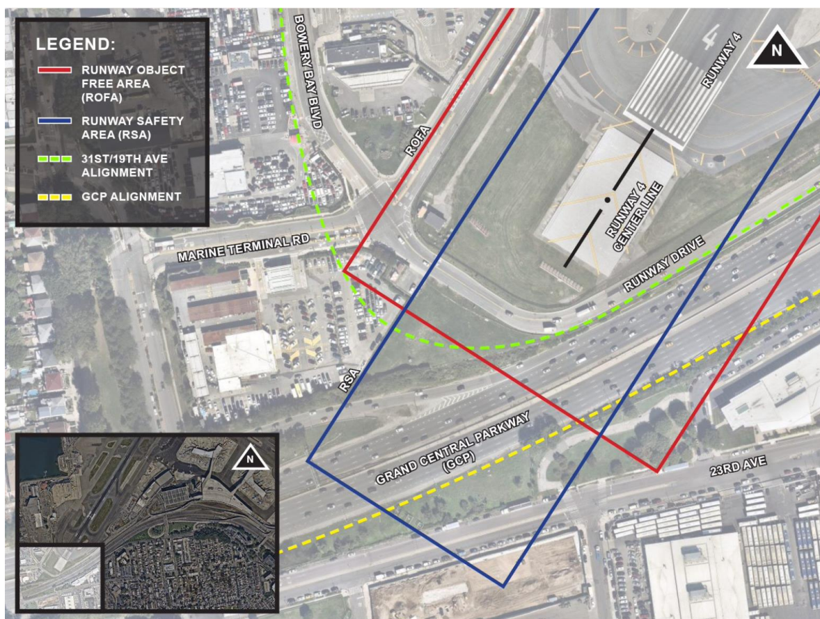
FIGURE 3.2-1: RUNWAY 04-22 PROTECTED ZONES AND IMPACTED OPTION ALIGNMENTS
